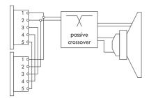
Fig. 4: Connector wiring
