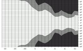
Fig. 10: Isobar diagram E8 vertical, horizontal setup with the horn rotated
