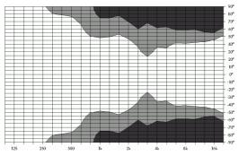
Fig. 9: Isobar diagram E8 horizontal, horizontal setup with the horn rotated
