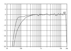
Fig. 11: E8 frequency response, standard and CUT settings
