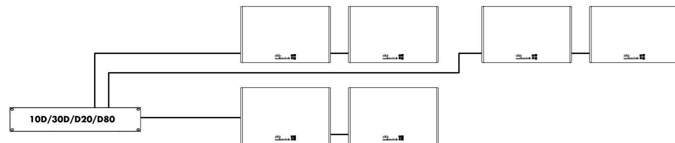
10D/30D/D20/D80 amplifier in mixed configuration with Dual Channel mode for MAX2, M6, M4 and 2-Way Active mode for M6 and M4
